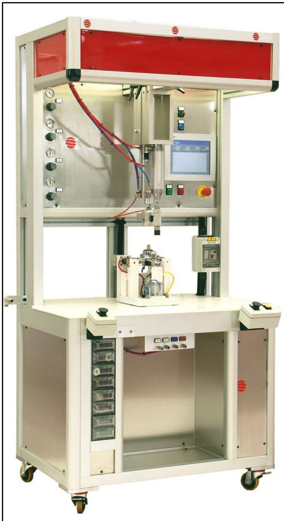
Semiautomatic bench for micro leaking seal test
