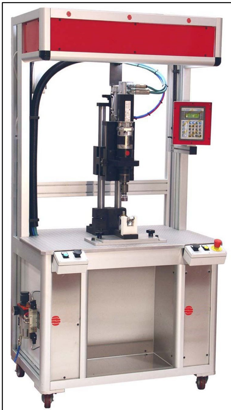
Assembly bench for cartridge locking
