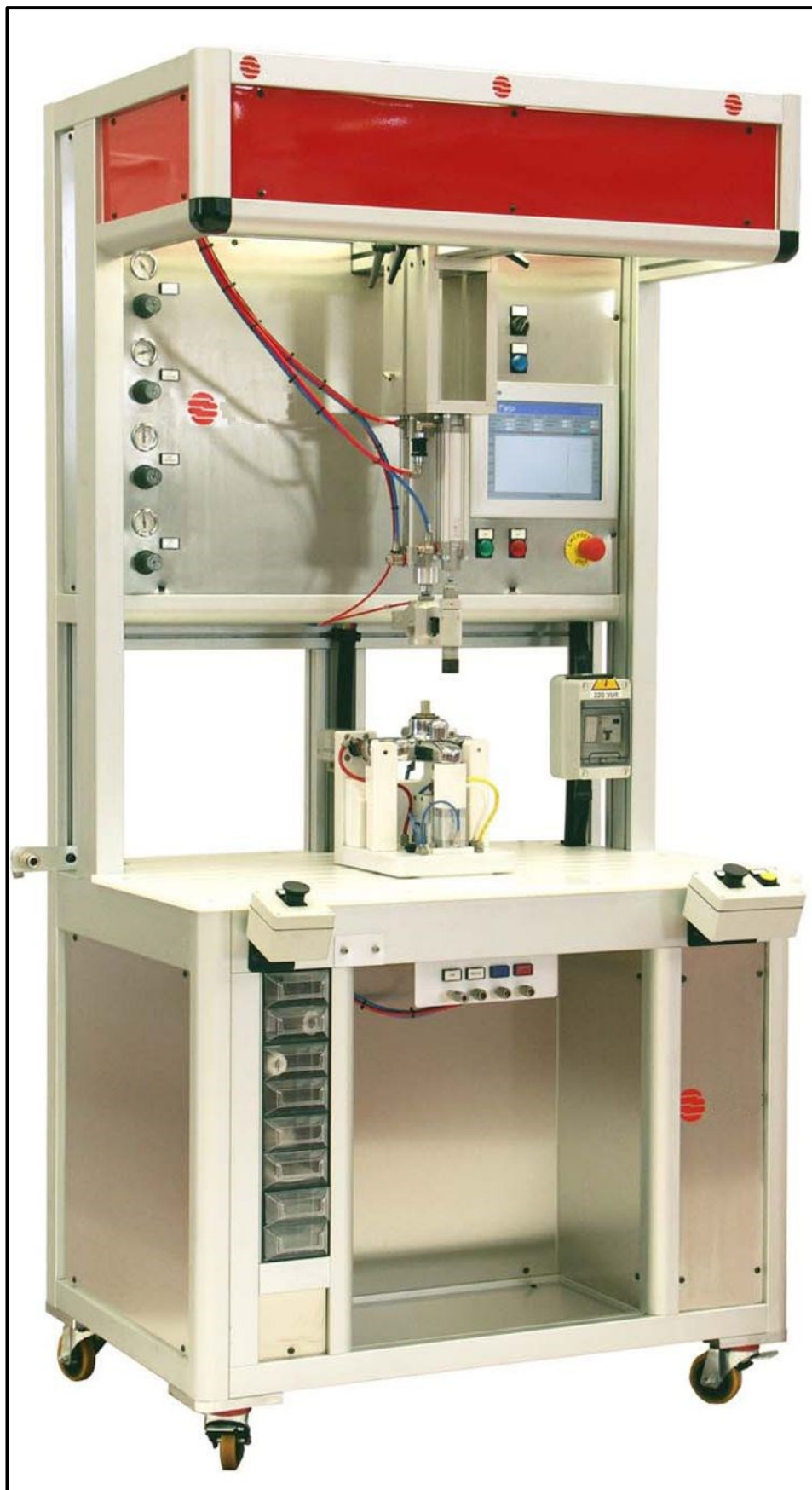
Semiautomatic bench for micro leaking seal test
