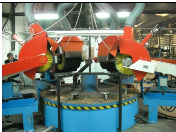
CONTINUE ROTARY TABLE WITH IMMERSION WORKING BUFFS TRC10/4
