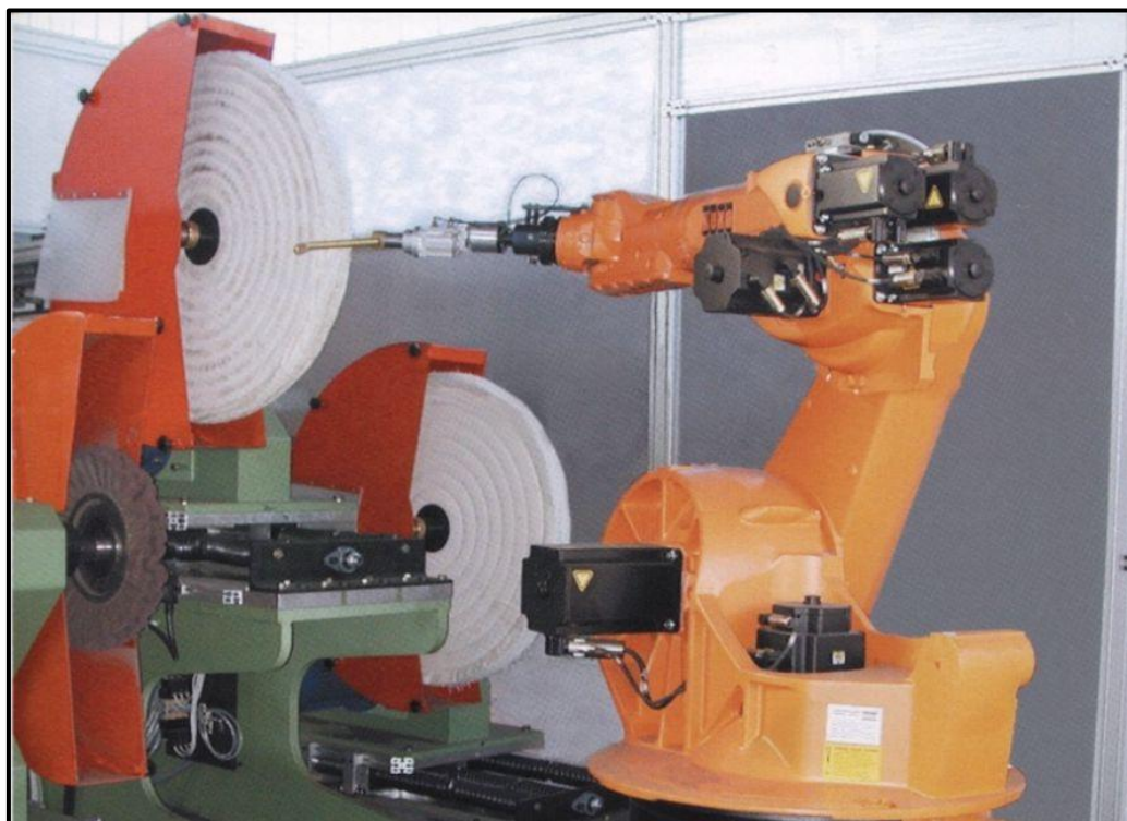
Station equipped with 2 robots for grinding working together or independently
