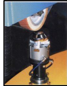
Rotary table machine For polishing or grinding
