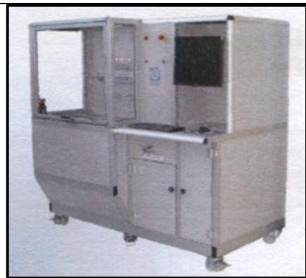
Hydraulic seal test with 100 bar maximum operating pressure;
