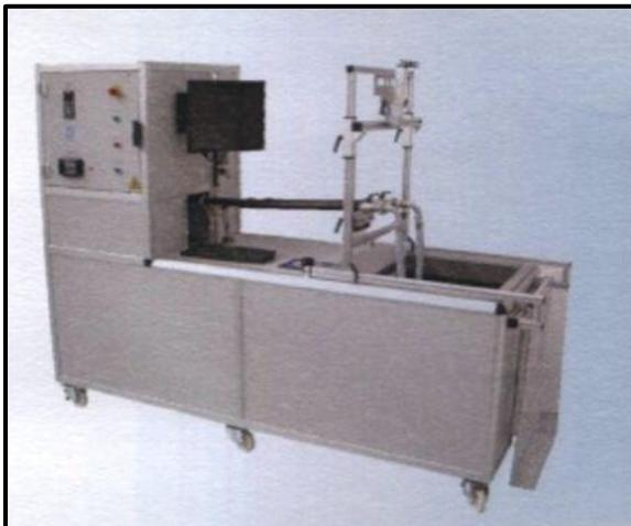
Noise tests performed in compliance with standard NF31-014 annex-C, test rig is designed according to ISO 3822 Standards;
