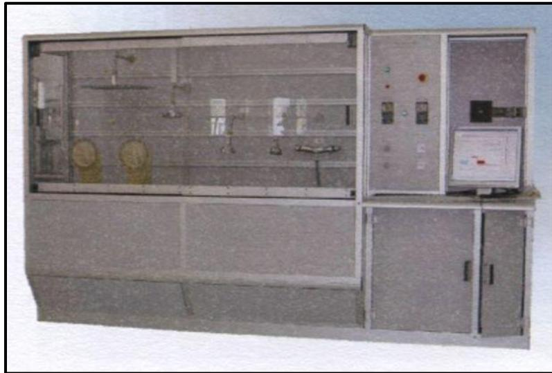
The bench performs tests to detect the hydraulic and thermal shock features on complete shower units, flexibles hoses, shower columns, diverters and accessories.
