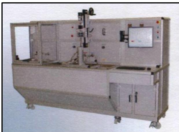
Complete version suitable to detect the hydraulic performance of the devices under test;
